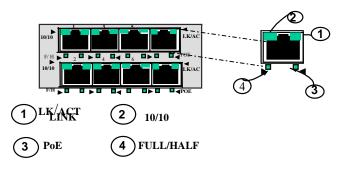
per the IEEE802.3af PoE standard. The Power Pass-through PoE modules are totally dependent upon the powerful -48VDC input power supply to support more RJ-45 (10/100) ports. Each port requires atleast 15watts to power up the PoE PD devices. Maxm. one PoE modules can be configured in the A, B slot of any 6K16 s with -48vdc power input. The PoE modules are also
